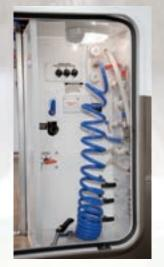
Docking Station includes outside shower, black tank flush, water bypass, 12V battery disconnect, selector switches, dump valves, water tank and city fills for centralized convenience.
