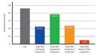
Compare acceleration forces experienced by an axle and trailer while traveling over railroad tracks at 30 MPH. The E-Z Flex® *System provides up to an 80% reduction in forces on the* trailer frame vs. a standard equalizer. E-Z Flex<sup>®</sup> significantly outperforms all other competitors in the same road test for a smoother, more protective ride for your trailer and cargo.
